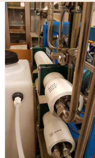
A photograph of the back showing two vessels for testing commercial module in parallel with SRI PBI HFMs
